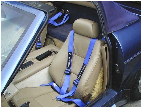
Fitted 4 point Willans harness.
